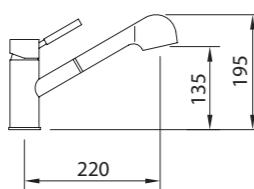
Mezclador con aireador, caño giratorio, flexibles M-10 3/8" x 370 mm. Mixer with aerator, swivel spout, flexible hoses M-10 3/8" x 370 mm. Mitigeur évier béc orientable, aérateur, raccords flexibles M-10 3/8" x 370 mm.
